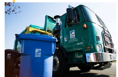
A hydraulic hybrid garbage collection truck consumes 33% less fuel than a traditional garbage truck
